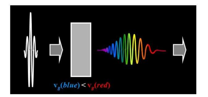
Because short pulses have such large ranges of wavelengths, GVD is a bigger issue than for nearly monochromatic light.
