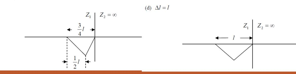
An incident wave travelling from a high density (low wave speed) region towards a low density (high wave speed) region. An incident wave travelling from a low density (high wave speed) region towards a high density (low wave speed) region.
