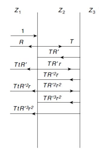
2. The relation between the impedance Z and the refractive index n of a dielectric is given by Z = 1/n. Light travelling in free space enters a glass lens which has a refractive index of 1.5 for a free space wavelength of  $5.5 \times 10^{-7}$  m. Show that reflections at this wavelength are avoided by a coating of refractive index 1.22 and thickness  $1.12 \times 10^{-7}$  m.
