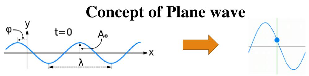
A typical representation of a wave propagating in space
