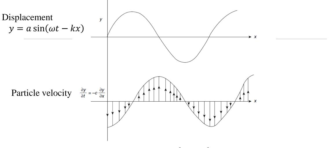
The magnitude and direction of the particle velocity  $\frac{\partial y}{\partial t} = -c \frac{\partial y}{\partial x}$  at any point x is shown by an arrow in the right-going sine wave above
