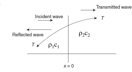
Waves on a string impedance  $\rho_1 c_1$  reflected and transmitted at the boundary x = 0 where the string changes to impedance  $\rho_2 c_2$
