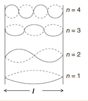
•Show that the total energy of the *n*th normal mode of a standing wave with a length of *l* is given  $E_n = \frac{1}{4}m\omega_n^2(A_n^2 + B_n^2)$
