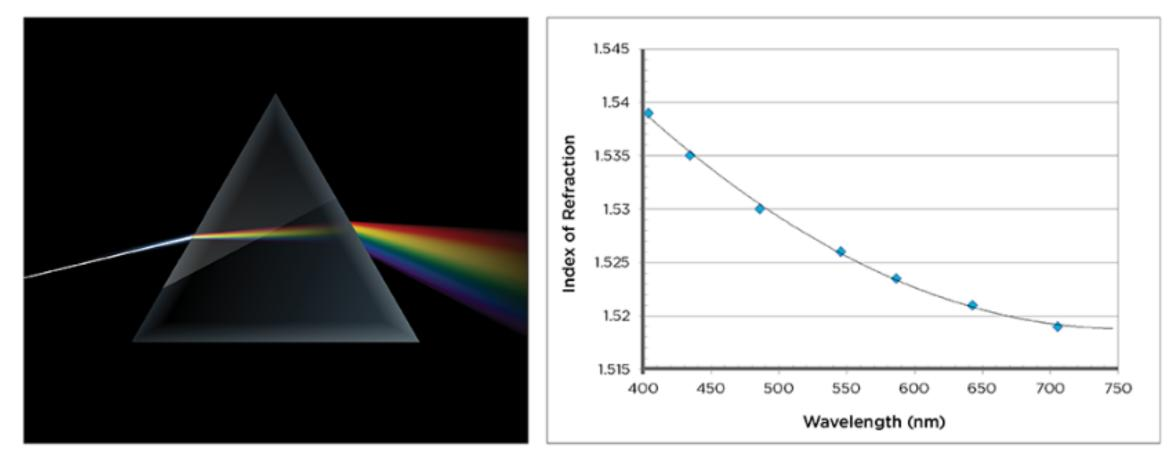
The index of refraction for a glass material changing over the visible wavelength spectrum. The use of an optical prism shows the effect of this change index across the visible spectrum as white light is split into individual wavelengths and colors.
